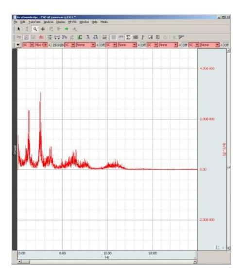
Most frequencies situated between 1 and 18 Hz => low pass 20 Hz [FIR: Blackman -91 dB/slope]
